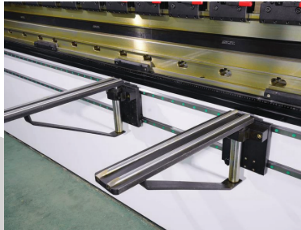
FRONT SUPPORTS WITH DUAL LINEAR GUIDE RAIL
