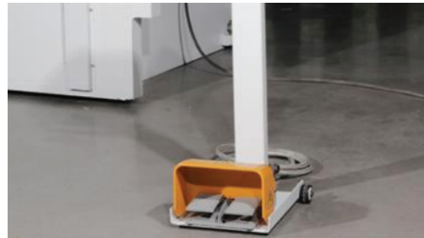
MOVABLE PEDAL SWITCH STATION WITH EMERGENCY STOP BUTTON
