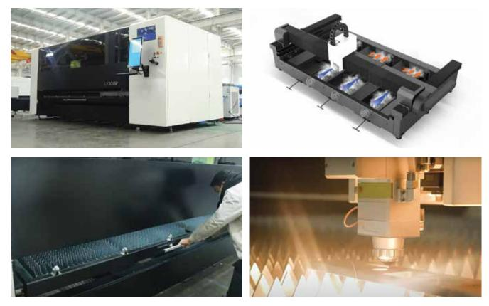
"Highlighting above the compact all-in-one design, 90degree orientation of the gantry with longer X axis, allowing for faster overall production. High pressure extraction through the frame tracking the head which allows for optimal extraction, pull-out table design and Raytools precision cutting head."
