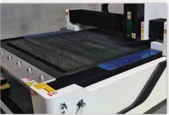
"Highlighting above the compact built in electrical cabinet with fan cooling, easy loading from any side, ball rollers on front side and 180degree pivoting control screen arm, with portrait style large control screen."
