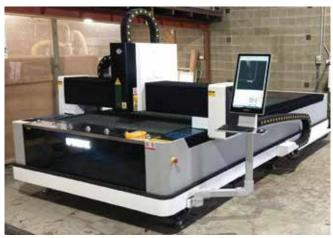
"Compact built in electrical cabinet with fan cooling, which can be moved to suit your factory set-up. Heavy Duty Hiwin guide rails and YYC rack sitting below the bed for easy loading."
