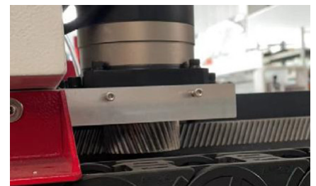
Metal Reinforced Belt, Dual Rack/Pinion, Simple Precision Head
