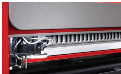
Dedicated Extraction Port/Fans For Each Zone
