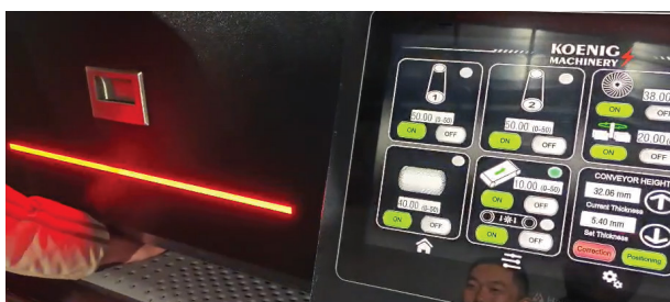
(From top left clockwise) User friendly touch screen controller, internal machine image, finished part as it exits the machine, safety interlock as side door opens, safety stop as hand enters the machine, part before finishing.
