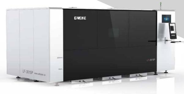
"The LF3015P Pro is our new 3000x1500mm bed size machine, with slide-out table. This innovative design allows for a fully enclosed large-formal bed size with minimal footprint in your factory floor. With slide out table, this machine can be easily loaded by overhead crane, jib-crane, forklift or by hand. The sliding table magnetically locks into place, with electronic closing access door for the ultimate safety enclosure."
